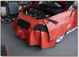
MG printed universal PVC Wing Cover with anti-slip foam backing and velcro fixing straps (MG18P) ~ MG printed semi tailored PVC front cover with solid blue foam anti-slip, ventilation mesh and adjustable fixing hooks (MG18TF)
