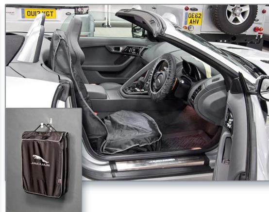
Re-Usable Technician's Kit, comprising: a Recaro style nylon seat covers, a rubber floor tray & a nylon steering wheel cover, all contained in a nylon kit bag for easy storage
